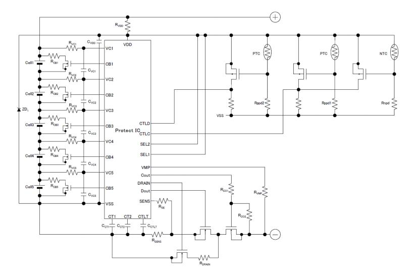
Partial circuit of temperature protection
