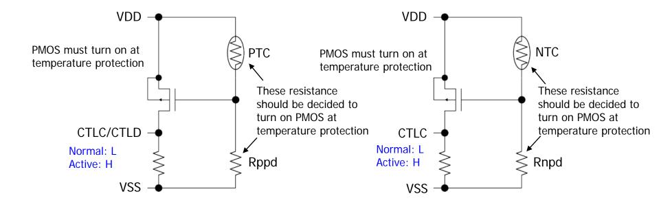
COUT(DOUT) turns off when CTLC(CTLD) is inputted VDD voltage
